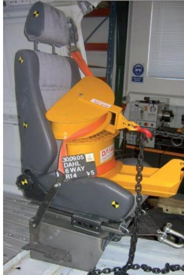
Figure 2-2: Seat belt anchorage test setup showing yellow traction devices.
